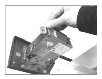
Feed the tickets into the mech, making sure that the ticket passes through the sensor.
