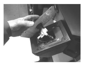
Remove the microswitch by unclipping it from the Lamp Housing
