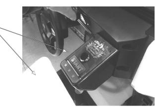
Once the Button plate has been removed to reveal the Switch and Lamp housing take care as not to pull on the assembly as damage to the harness may occur.
