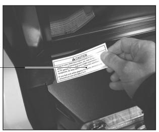
Apply the label to the top left hand corner of the Control Panel. This location is unobstructed and can be easily read by players and observers alike.
